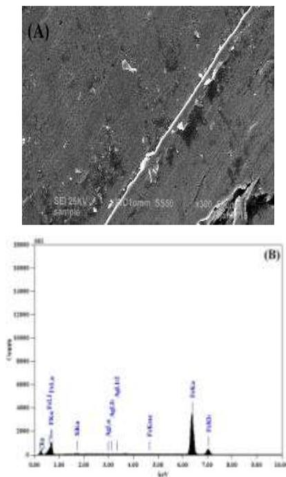
**Figure 8:** (A) SEM image of the wear formed on the pin lubricated with grease+AgNPs (L1), (B) EDX spectrum performed on wear on the pin lubricated with grease+AgNPs (L1).
