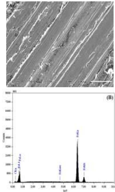
**Figure 7:** (A) SEM image of the wear formed on the pin lubricated with lubricating grease (L), (B) EDX spectrum performed on wear on the pin lubricated with lubricating grease (L).
