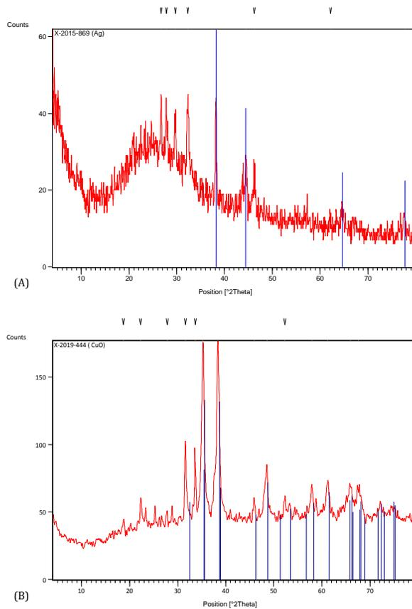
**Figure 5:** (A) XRD of Silver nanoparticles (AgNPs), and (B) XRD of Copper oxide nanoparticles (CuO- NPs).
