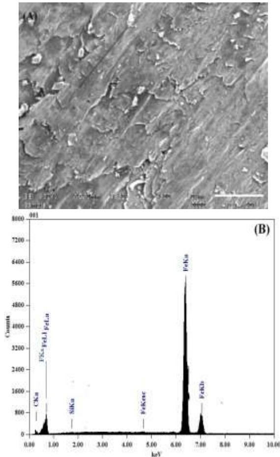
**Figure 6:** (A) SEM image of the wear formed on the blank pin (metal to metal), (B) EDX spectrum performed on wear on the blank (metal to metal).
