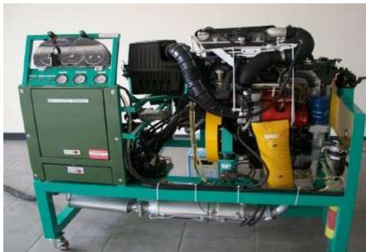
**Figure 1:** Experimental set-up of the diesel engine testing system.
