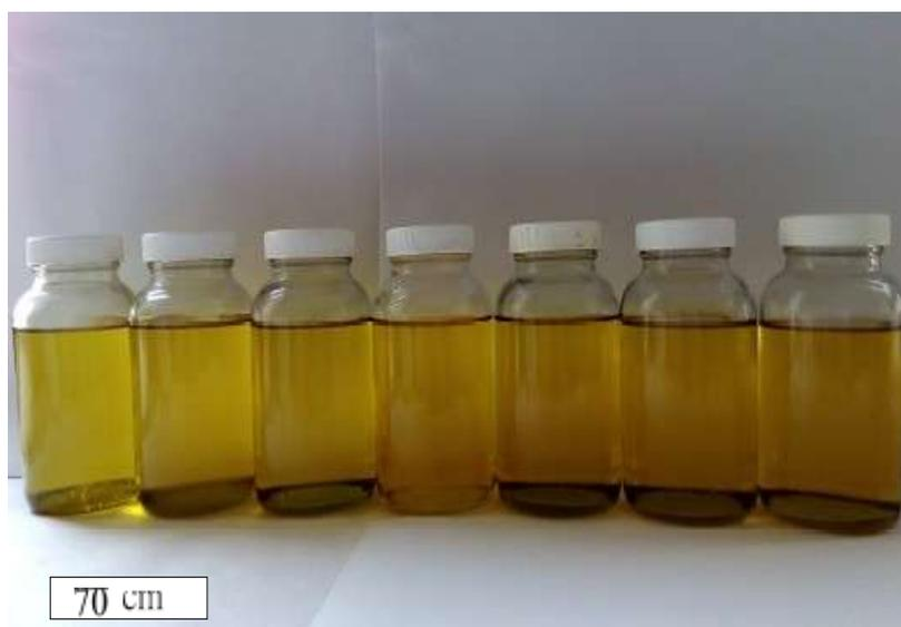
**Figure 2:** The sedimentation of biodiesel in petro-diesel of pure petro-diesel (left), 2% biodiesel, 5% biodiesel, 10% biodiesel, 20% biodiesel, 50% biodiesel and 100% biodiesel (right).
