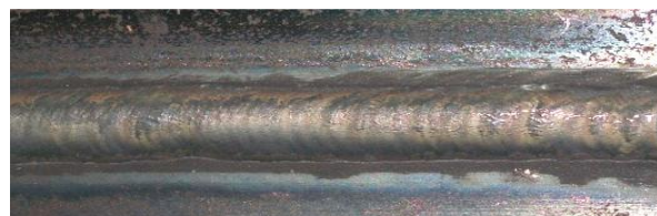
Figure 4: Morphology of the GTAW-clad coating
