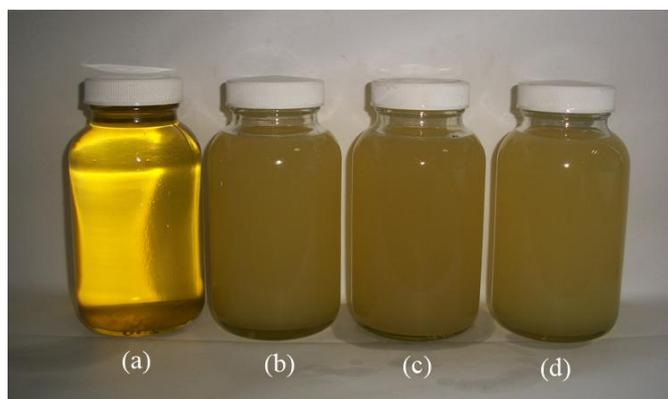
**Figure 2:** Sedimentation of methanol in (a) pure ultralow sulfur diesel, and pure ultralow sulfur diesel blended with (b) 1 wt.% methanol, (c) 2 wt.% methanol, and (d) 5 wt.% methanol.
