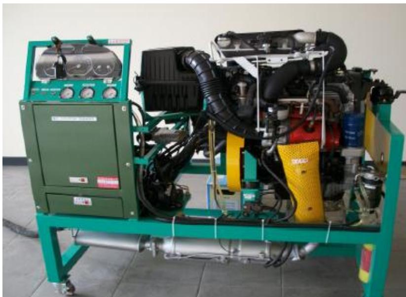
**Figure 1:** Experimental set-up of the diesel engine testing system.
