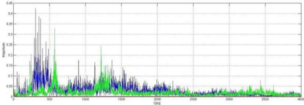
**Figure 1:** Vibration acceleration spectrum; the vehicle moved on tarmac surface with a velocity of 37 km/h; blue colour – acceleration value measured on the engine's body, green – on the driver's seat, red – on the driving axle.
