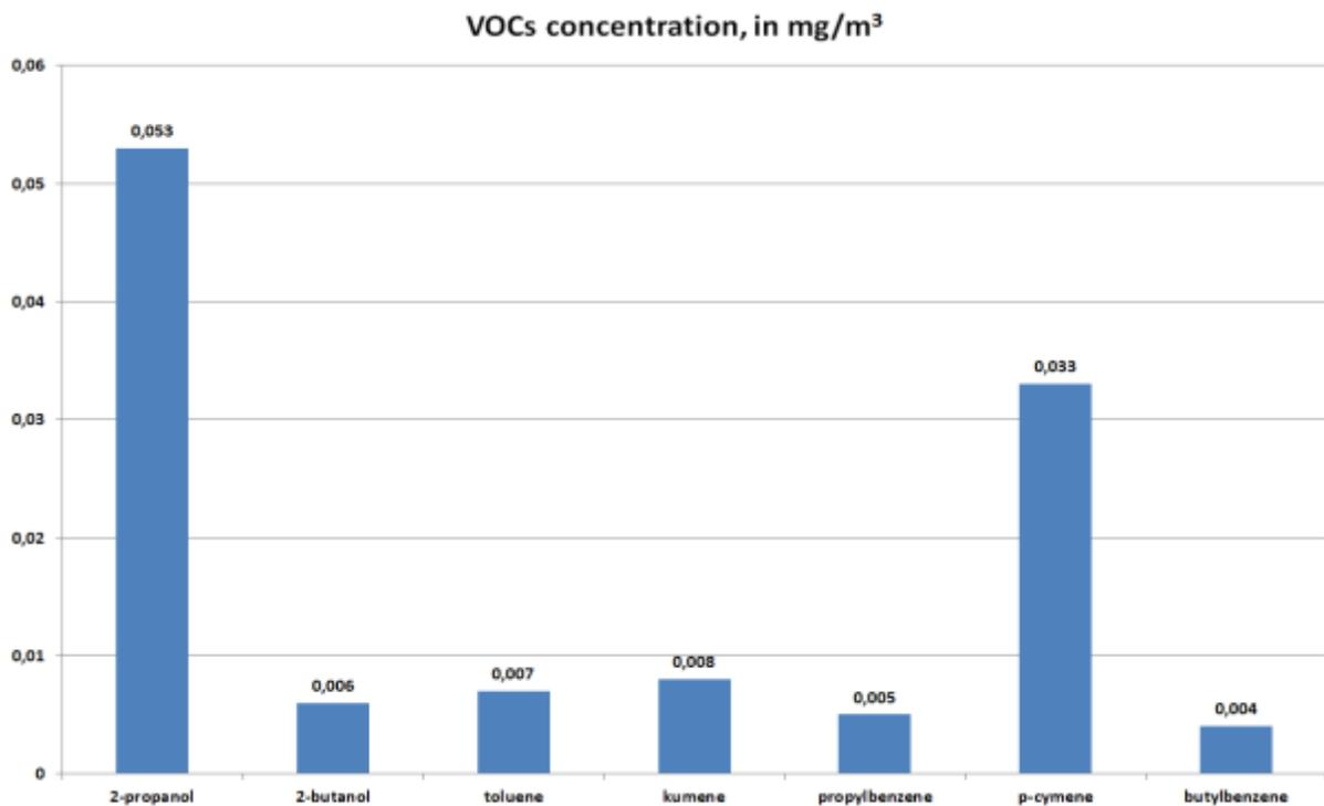
**Figure 1:** Concentrations of volatile organic compounds identified inside the tractor's cabin.
