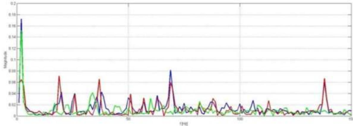
**Figure 5:** The Frequency domain of acceleration (tarmac, 31 km/h) measured on the driver's seat; blue – in solitary, red – the tilling set, green – the trailer.
