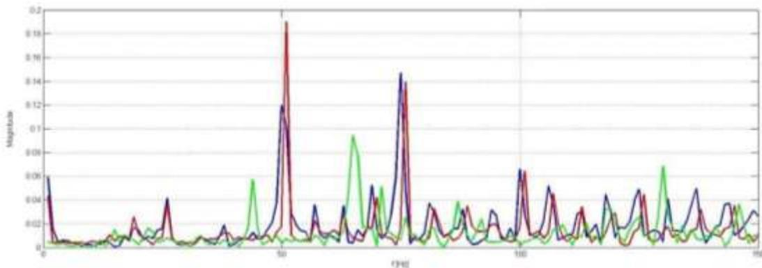
**Figure 4:** The Frequency domain of acceleration (tarmac, 31 km/h) measured on the engine's body; blue - in solitary, red - the (generator) tilling set, green - the trailer
