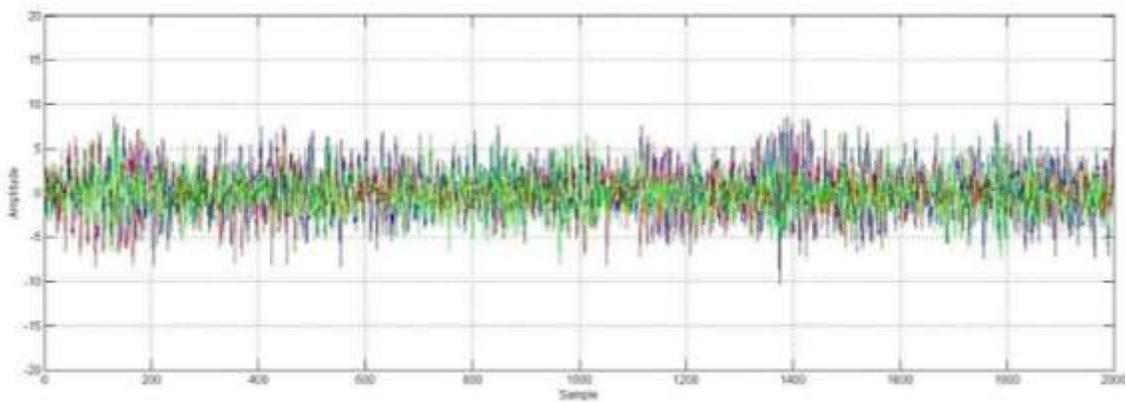
**Figure 3:** Time domain of vibration (tarmac, 31 km/h) measured on the driver's seat; blue - in solitary, red - the (generator) tilling set, green - the trailer.
