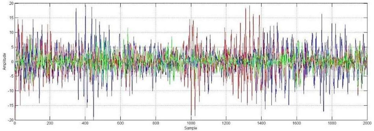
**Figure 2:** Time domain of vibration (tarmac, 31 km/h) measured on the engine's body; blue - in solitary, red - the (generator) tilling set, green - the trailer.
