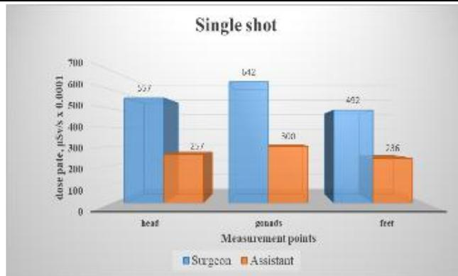
**Diagram 1:** Average values recalculated for the dose rate, received for the operator and his assistant using radiography mode (single shot).
