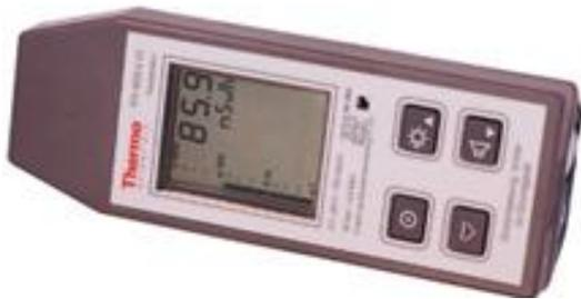
**Figure 2:** FH 40 G-L multi-purpose digital survey meter.
