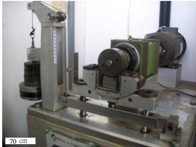
**Figure 2:** TE-53 wear test rig
