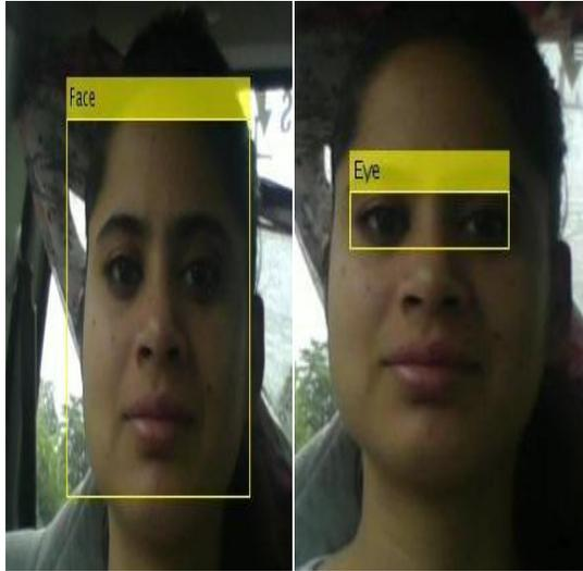
**Figure 1:** Multi-stage approach for eye centre localisation. A face detector is applied first; based on the face location rough eye regions are extracted (left), which are then used for a precise estimation of each eye centre (middle and right).
