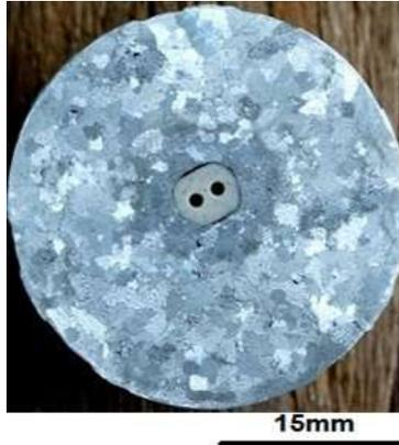
**Figure 2:** Test run 1 macrography: Addition of 0.15% (in wt.%) of TiB<sub>2</sub> in the bath.
